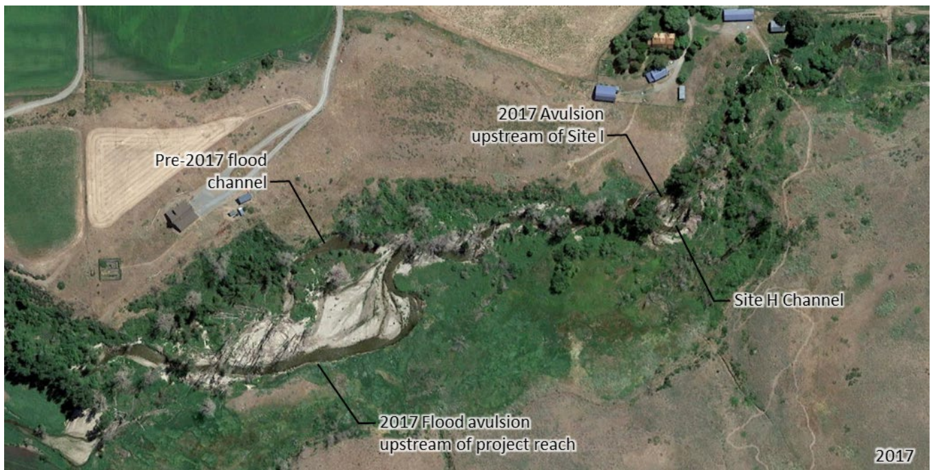
Figure 3-41. Aerial view of 2017 post-flood Beaver Creek channel conditions near Sites H and I.
