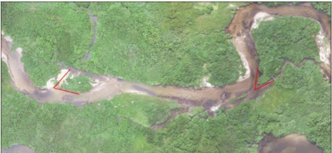
Figure 3-7. Example measurement of secondary channel inlet angle.
